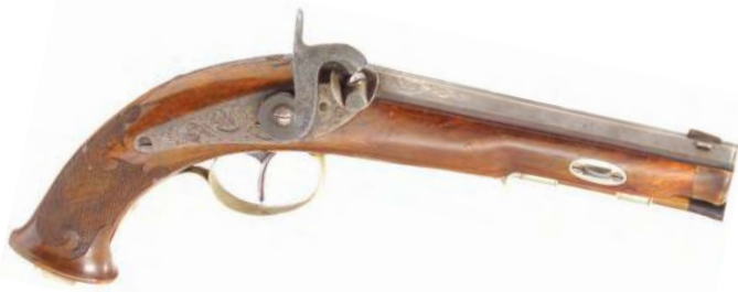
A 1830 caplock pistol with a muzzle velocity of 850 feet/second. INTERFOTO / Alamy Stock Photo
