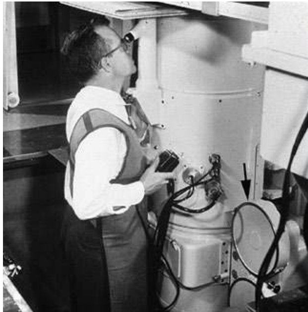
Mason Sones, MD, in the submerged pit looking up at an intensified image. The circular unit on the right is the 35-mm cine camera. Photo courtesy Cook Corporation
