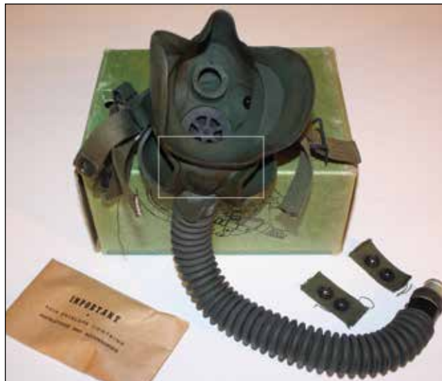
The inside of the A-14 aviation mask developed at the Mayo Clinic with Lindbergh's contribution. The white box demonstrates the relationship of the vents to the right and left of the pilot's mouth that were designed to remove water vapor. Carbon dioxide had to be removed by soda lime which can potentially cause lung damage. Courtesy of 303rd Bombing Group
